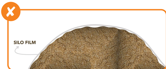
Inferior sheets causing air pockets
